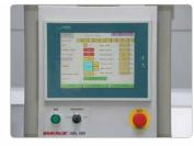
Operator-friendly, multi-language, touch screen control panel allows format changes to be made quickly and easily. The job memory function for the automatic storage of product settings is available as an optional extra.
