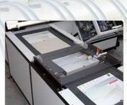
Optional extra: DBW 500 - conveyor flips the back cover into position.
