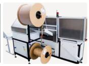
Spool de-winding with integrated paper separation re-winding
