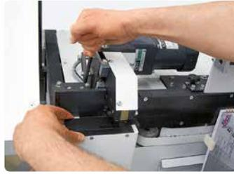
Diameter can be easily adjusted with interchangeable guide plates per diameter.
