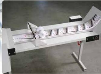
Optional extra: Shingle conveyor - height adjustable conveyor can be used in a continuous running function or with an adjustable overlap setting.
