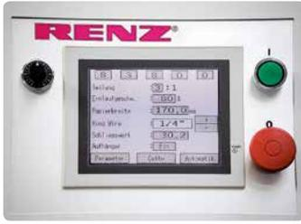
Operator-friendly touch screen control allowing very quick and easy format changes.
