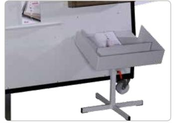
A standard catch tray collects the bound product. This can be upgraded with the optional shingle conveyor for quicker handling workflow.
