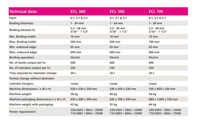
All performance outputs are based on 80 gsm paper and may vary depending on the product type, the working environment and the operator.
