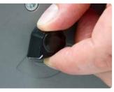
Depth gauge feature allows the operator to adjust the punched hole margin from 2 mm to 4,5 mm. This adds strength to the bound edge.
