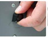
Depth gauge feature allows the operator to adjust the punched hole margin from 2 mm to 4,5 mm<sup>(1)</sup>. This adds strength to the bound edge.
