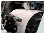
Turnover drum keeps the punched sheets in the correct page sequence and delivers them to the ejection system.
