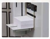
Deep pile feeder with high prestack capacity up to 4.000 sheets.
